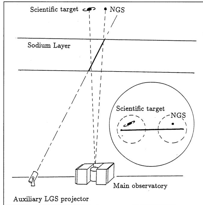
**Fig. 1.** A section of the method described in the text. In the circular inset the objects, as seen in the FoV of the main observatory, are sketched; the dashed circles represent the isoplanatic patch size.
