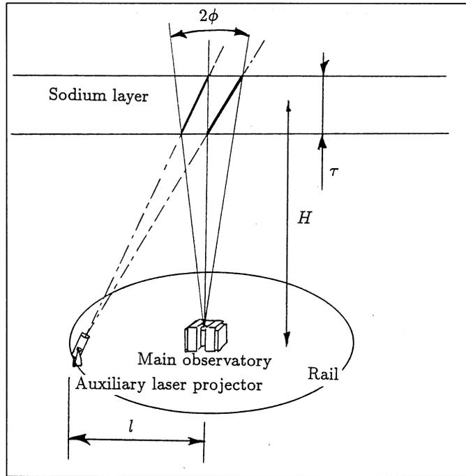
**Fig. 2.** The two auxiliary LGSs projectors should be movable in a circular track around the main observatory, with a radius  $l$  and spanning an angle of the order of 180deg.
