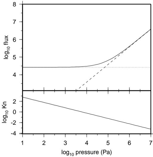
**Fig. 1.** Diffusion flux ( $\text{H}_2\text{O}$ ) of a binary gas mixture across a capillary (diameter  $1 \mu\text{m}$ ) at  $150 \text{ K}$  with constant pressure gradient. The gas is composed of  $\text{H}_2\text{O}$  (50 %) and  $\text{CO}$  (50 %). The 3 curves are obtained with the Poiseuille (viscous, dashed line) and Knudsen (free molecular, dotted line) formula as well as with the *Chapman-Enskog* method (solid line). For comparison the Knudsen number is plotted below.
