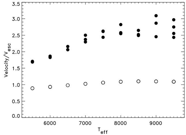
**Fig. 9.** The predicted ratio  $v_{\infty}/v_{\text{esc}}$  as a function of effective temperature for our models. Filled circles indicate our non-isothermal models with the  $CF$  correction. Open circles refer to Abbott's predictions for isothermal winds without the  $CF$  correction. The mean predicted ratio decreases from about 2.7 at 9000 K to about 1.7 at 5500 K.
