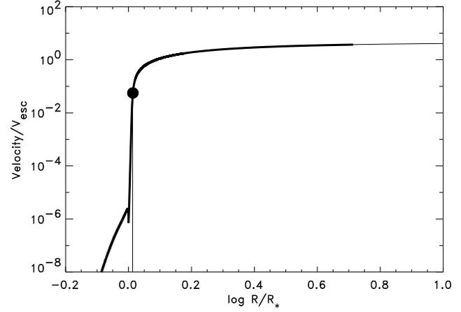
**Fig. 8.** The fitted beta-law velocity structure (thin line) compared to the calculated velocity structure (thick line). The values of  $\beta$  is 0.81 and the terminal velocity  $v_{\infty}$  is  $390 \text{ km s}^{-1}$ . Note that the dip at around  $R = R_*$  is due to the pressure inversion. The location of sonic point is marked by a filled circle.
