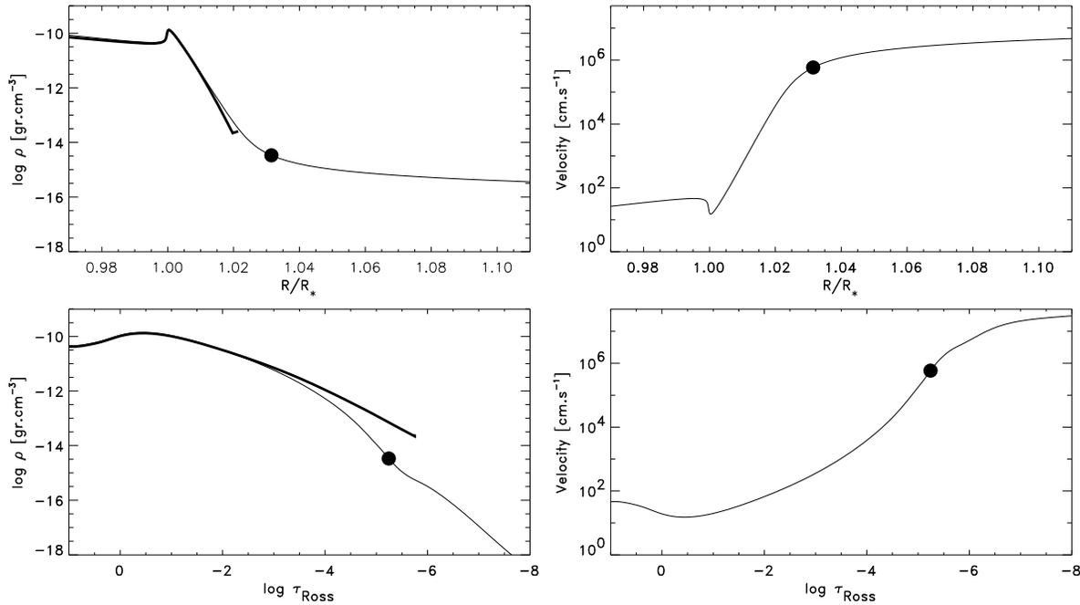
**Fig. 5.** The  $\rho(r)$  and  $v(r)$  as functions of radius and optical depth. The thick lines are the hydrostatic plane-parallel model and the thin lines are the hydrodynamic model. The filled circles are the location of the sonic point. Note that the stellar radius corresponds to  $\tau_{\text{Ross}}=2/3$ .
