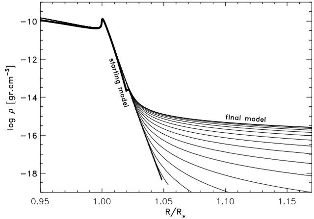
**Fig. 4.** The density structure of hydrodynamic models during the iteration. The thick-solid line, labeled as 'starting model', is the Kurucz's hydrostatic density structure. The other lines are the hydrodynamic solutions from the first until the last iteration, labeled as 'final model'.
