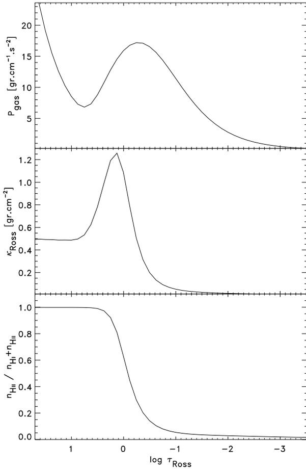
**Fig. 1.** The upper graph: the  $P$ -inversion of hydrostatic model of Kurucz with  $T_{\text{eff}} = 7500$  K and  $\log g = 0.5$ ; the middle graph: the Rosseland absorption coefficient ( $\kappa_{\text{Ross}}$ ) and the lower graph: the ionization fraction of hydrogen. Notice that the 'bump' in  $\kappa_{\text{Ross}}$  is related to the hydrogen ionization zone and that the peak of  $\kappa_{\text{Ross}}$  coincides with the steepest outward increase of  $P_{\text{gas}}$ .
