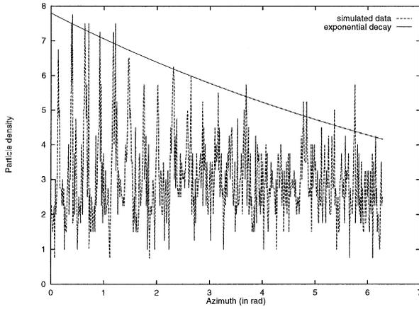
**Fig. 5.** Azimuthal section of the simulated ring in Fig. 4 near the edges of the gap showing the decay of the wake intensity after the passage of the moon. The strong fluctuations are due to the comparatively low number density of the particles. In order to reduce them, density values of points which are situated axisymmetric with respect to the moon have been summed. The solid line corresponds to a exponential decay of the density maxima according to  $I = 7.8 \exp(0.1 \cdot \phi)$ .
