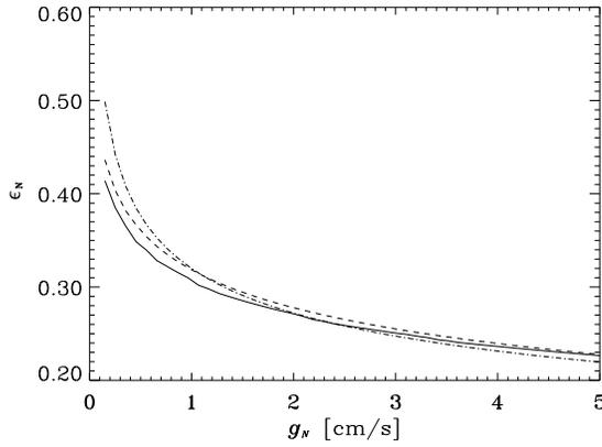
**Fig. 1.** Dependence of the normal restitution coefficient on the normal component of the impact velocity. Dash-dotted: experimental results (Bridges et al. 1984). Solid: theoretical results (Hertzsch et al. 1995). Dashed: theoretical results using a simplified model (Spahn et al. 1995).
