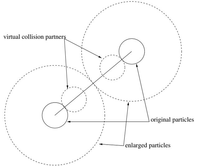
**Fig. 2.** The concept of "virtual particles": the radii of the particles are artificially enlarged in order to enhance the collision probability. After the detection of a collision, the simulation continues as if each particle had collided with another of the original size, but also at a distance which corresponds to the sum of the radii of the original and the "virtual" particles.
