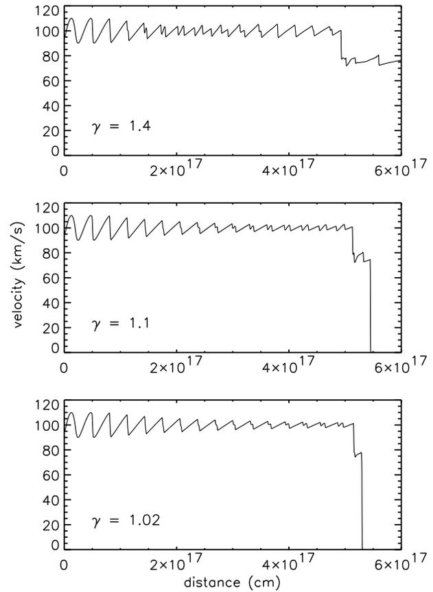
**Fig. 1.** One-dimensional pulsed jets. The velocity patterns for three specific heat ratios are shown. The jets ( $10^5 \text{ cm}^{-3}$ , ten times the ambient density) propagate over  $5 \cdot 10^{17} \text{ cm}$  at the time 2159 years of these snapshots. Note how the pulse development depends on  $\gamma$ .
