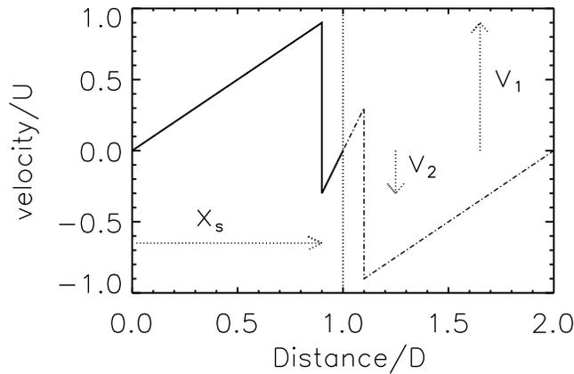
**Fig. 5.** Isolation of a pulse and the reduction of the flow problem employing the symmetries observed in the slowly-evolving pulses displayed in Figs. 1 and 2. Note the pulse wavelength is  $\lambda_p = 2D$ .
