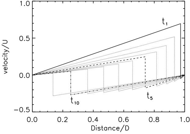
**Fig. 6.** The time sequence for the pulse velocity structure with  $\gamma = 1.1$  obtained via the analysis. Each tooth is separated by a time  $0.2 D/U$ , from the solid line ( $t_1 = 0.2 D/U$ ), through the dash ( $t_5 = D/U$ ) to the dot-dashed line at  $t_{10} = 2D/U$ . Note that the sawtooth amplitude, shock jump and velocity gradients all decrease with time.
