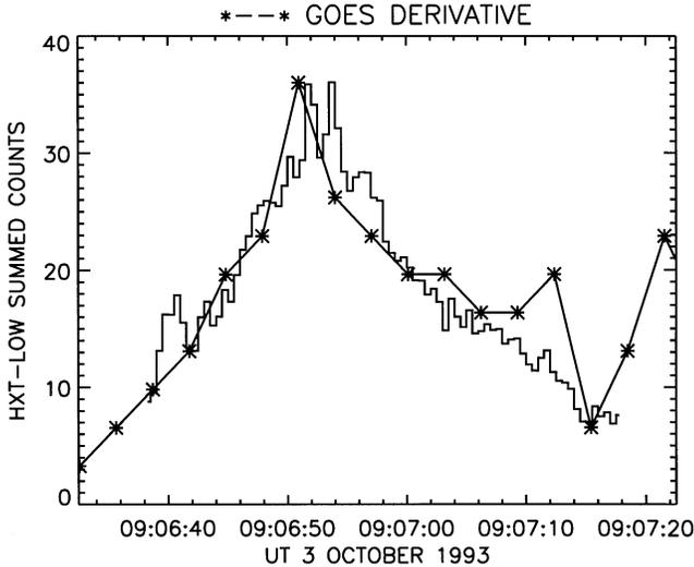
**Fig. 3.** High-resolution view of the Neupert effect in the first spike: comparison of the HXT 15–23 keV counting rate (plus signs) at 0.5 sec resolution, with the time differences of successive GOES soft channel (2–8 Å) data (asterisks). Within the time resolution of the latter, there is no perceptible advance or delay.
