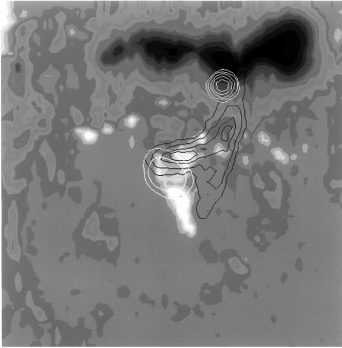
**Fig. 9.** Overlay of soft X-ray (black contours) and HXT (white contours) on a high-resolution magnetogram from Kitt Peak National Observatory, rebinned to SXT resolution. We estimate the accuracy of the overlay at one SXT pixel ( $2.46''$ ). The north hard X-ray footpoint lies in a region with more magnetic flux (see text). It continues to have much higher surface brightness throughout the successive bursts.
