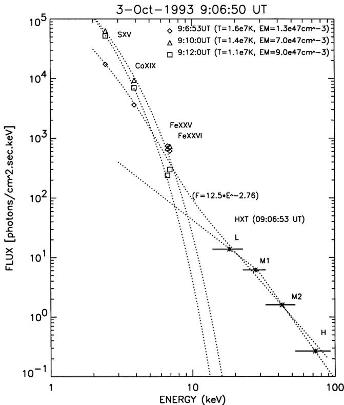
**Fig. 5.** Continuum spectra inferred from the *Yohkoh*/BCS and *Yohkoh*/HXT total counting rates, during the evolution of the initial flat-spectrum burst. The four HXT channels have been fitted to a broken power law (low-energy index  $1.98 \pm 0.04$ ; high-energy index  $3.34 \pm 0.03$ ), as well as with a single power law (index  $2.76 \pm 0.01$ ). The impulsive source seen in the BCS counters lies somewhat above the extrapolation downwards from the HXT energy range in the two-power-law fit.
