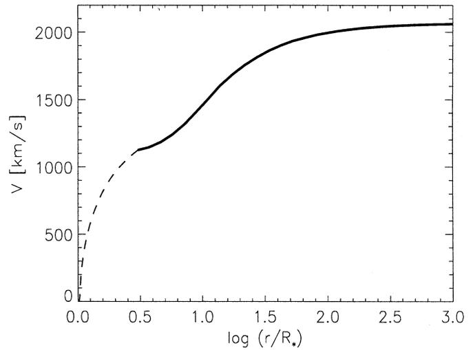
**Fig. 10.** The velocity structure of the final model. The hydrodynamically calculated velocity law is shown by the full drawn line, the assumed velocity law in the optically thick atmosphere is illustrated by the dashed line.
