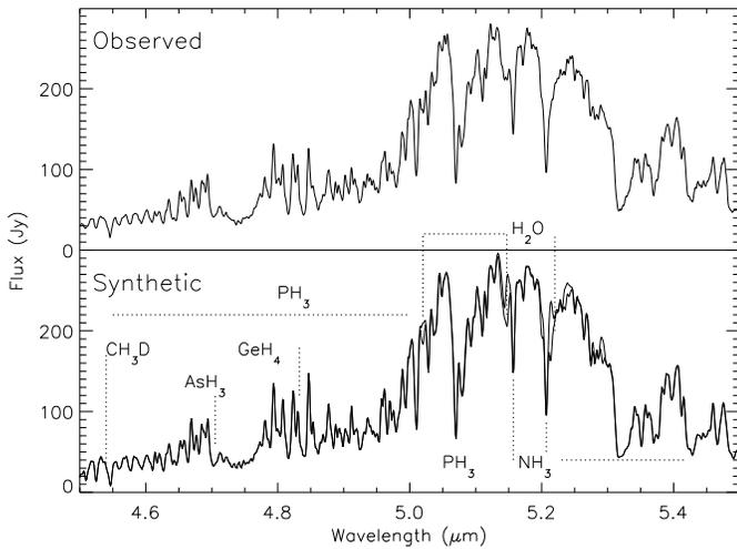
**Fig. 1.** Observed ISO-SWS spectrum (upper curve) and synthetic spectrum of Saturn (lower curve) in the 5- $\mu\text{m}$  region. Spectral absorptions are due to  $\text{NH}_3$ ,  $\text{PH}_3$ ,  $\text{AsH}_3$ ,  $\text{GeH}_4$ ,  $\text{CH}_3\text{D}$  and  $\text{H}_2\text{O}$ . In the lower curve, the narrow line corresponds to a calculation without  $\text{H}_2\text{O}$ .
