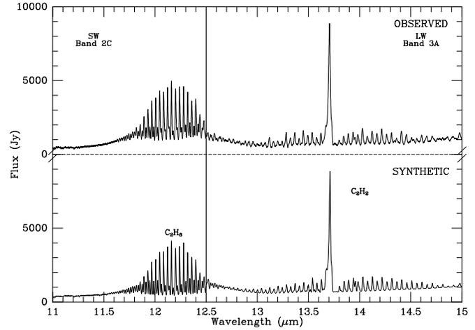
**Fig. 3.** Observed ISO-SWS spectrum of Saturn (upper curve) and synthetic spectrum (lower curve) between 11 and 15  $\mu\text{m}$ . Molecular emissions are due to  $\text{C}_2\text{H}_6$  and  $\text{C}_2\text{H}_2$ .
