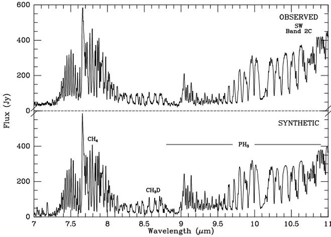
**Fig. 2.** Comparison between the Saturn ISO-SWS data (above) and a synthetic model (below) in the 7–11  $\mu\text{m}$  range. The spectrum shows stratospheric emission features due to  $\text{CH}_4$ , and tropospheric absorption features due to  $\text{CH}_3\text{D}$ ,  $\text{PH}_3$  and  $\text{NH}_3$ .
