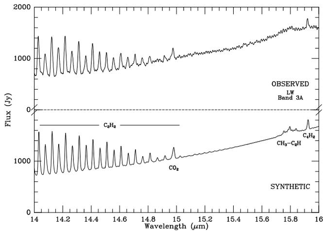
**Fig. 4.** Observed ISO-SWS spectrum of Saturn (upper curve) and synthetic spectrum (lower curve) between 14 and 16  $\mu\text{m}$ . The 14.98  $\mu\text{m}$  emission feature is attributed to  $\text{CO}_2$ . Emission from  $\text{C}_4\text{H}_2$  (15.92  $\mu\text{m}$ ) and  $\text{CH}_3\text{-C}_2\text{H}$  (around 15.8  $\mu\text{m}$ ) are also detected. Below 15  $\mu\text{m}$ , lines from the P-branch of the  $\nu_5$  band of  $\text{C}_2\text{H}_2$  dominate the spectrum.
