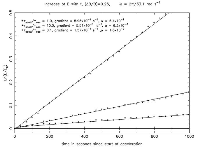
**Fig. 2.** The increase of energy with time by homogeneous magnetic pumping in the non-relativistic regime, for 3 values of the pitch-angle scattering to field oscillation time. The straight lines are fits to the numerical data, given by the points.  $\alpha$  is calculated given the field parameters indicated.
