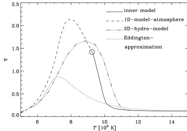
**Fig. 2.** Temperature gradient  $\nabla = \frac{d \ln T}{d \ln P}$  of the models shown in Fig. 1. Only the superadiabatic temperature range is shown.
