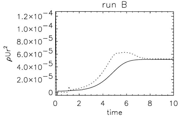
**Fig. 2.** Wind formation; mass flow  $F = \rho u r^2$  through the bottom (continuous) and top (dotted) of the domain versus time (run B).
