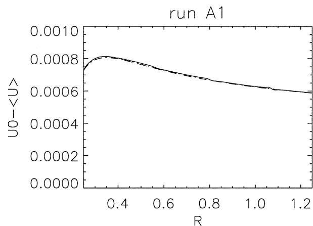
**Fig. 5.** Mean velocity variation due to the waves (run A1). (continuous) simulation result; (dotted) using Eq. (17b); (dashed) using Eq. (17a).
