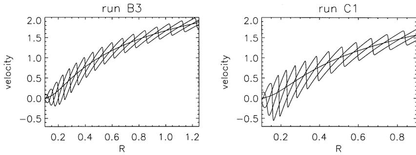
**Fig. 14.** Unperturbed and perturbed velocity profiles **a** run B3 **b** run C1.
