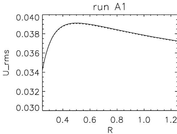
**Fig. 4.** Profile of rms wave amplitude  $\delta u_{\text{rms}}$  (run A1). (continuous) simulation result (dotted) Linear extrapolation of the wave profile from the inlet amplitude, using the WKB Eq. (5b).
