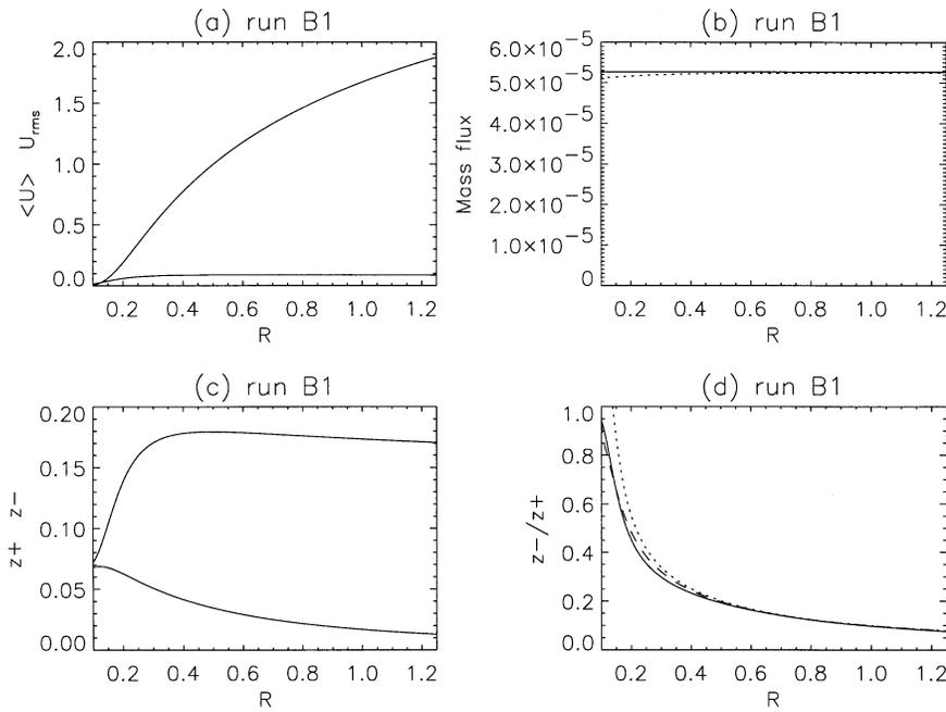
**Fig. 7a-d.** Averages and rms values, run B1. **a** Mean and rms velocity profile **b** Mean mass flux  $\langle F \rangle = \langle \rho u r^2 \rangle$  (continuous) and partial contribution  $F^\circ = \langle \rho \rangle \langle u \rangle r^2$  (dotted) **c** rms amplitudes  $z^+$  and  $z^-$  **d** ratio of rms amplitudes  $z^-/z^+$  (continuous: simulation; dotted: linear approximation (Eq. (4))  $z^-/z^+ = -i\varepsilon$ ; dashed: full Eq. (4)).
