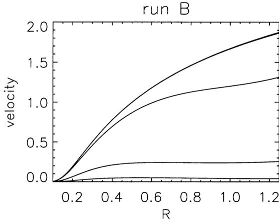
**Fig. 1.** Transonic wind formation by perturbation of a static atmosphere; successive radial profiles of the velocity at times  $T = 0, 2, 4, \dots, 12$ . (run B,  $0.1 \leq r \leq 1.25$ ). The sonic point is at  $r = 0.5$  (see text).
