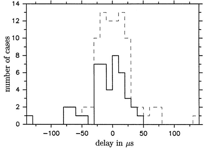
**Fig. 3.** The delay of 45 model spikes was measured in artificial, noisy model spikes (cf. Eq. 1) having an input delay of  $\tau = 0$ . The full histogram shows the number of cases per 25  $\mu\text{s}$  bin. The dashed histogram is the distribution neglecting the sign of the delay.
