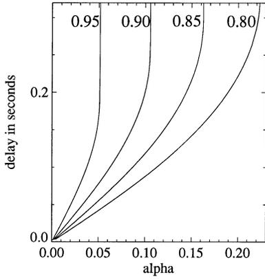
**Fig. 5.** Time delay between circular modes as a function of  $\alpha = \Omega_e |\cos \theta| / \omega_p$  for various starting values  $X_0$  indicated in the figure ( $X_0 = \omega_{p0}^2 / \omega^2$ ). A density scale height of  $H_n / \cos \Phi = 10^{10}$  cm has been assumed.
