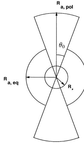
**Fig. 1.** Sketch of the considered geometry.  $R_*$  is the stellar radius and  $R_A$  the Alfvén radius. We distinguish between the polar regions, with  $R_A = R_{A,\text{pol}}$ , and an equatorial ring with  $R_A = R_{A,\text{eq}}$ . The angle  $\theta_0$  marks the co-latitude of the boundary between the two parts of the stellar surface
