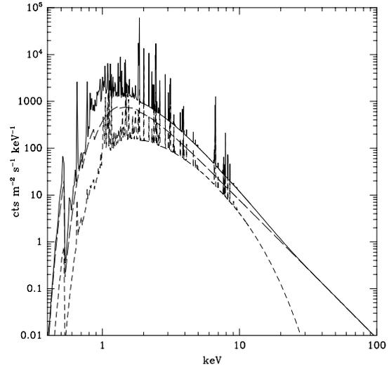
**Fig. 2.** The deconvolved broad-band BeppoSAX spectrum of Cas A, using the data from the LECS, MECS, HPGSPC and PDS, together with the individual contribution from the best-fit two-component NEI model and the power-law high energy tail.
