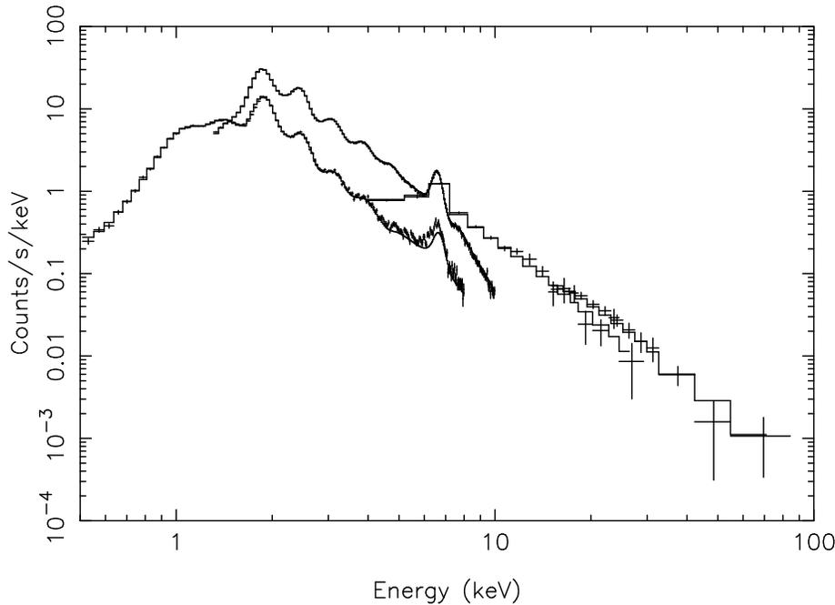
**Fig. 1.** The observed composite BeppoSAX spectrum of Cas A, using data from the LECS, MECS, HPGSPC and PDS instruments, together with the best-fit two-component NEI plus power-law model.
