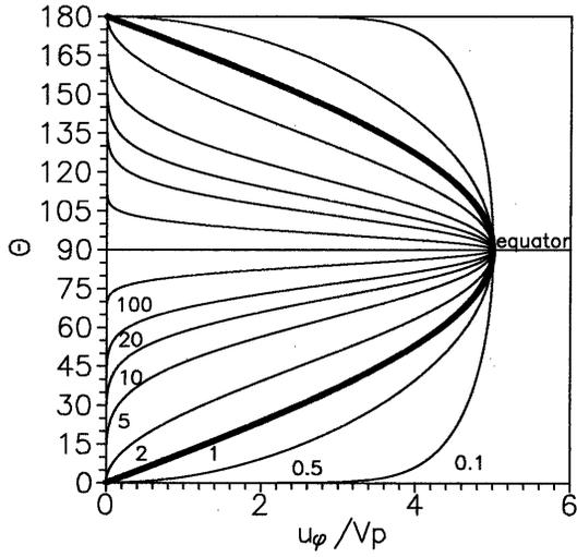
**Fig. 1.** Differential fluid rotation described by Eq. (5). The dependence of the dimensionless azimuthal velocity upon the colatitude  $\theta$  at the stellar surface for several values of the exponent  $\mu$  ( $\mu = 0.1, 0.5, 1, 2, 5, 10, 20, 100$ ). Increasing  $\mu$  steepens the fluid rotating area close to the equatorial plane.
