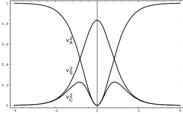
**Fig. 1.** Profiles of the characteristic speeds (squared): the Alfvén  $v_A^2(x)$ , the sound  $v_s^2(x)$  and the cusp  $v_C^2(x)$ .
