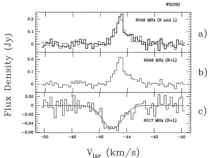
**Fig. 7a–c.** The 6 GHz OH satellite lines. In **a** the ( $F = 3 - 2$ ) 6.049 GHz line ( $RC$  heavy,  $LC$  light contours). In **b** the sum of  $RC$  and  $LC$  for the 6.049 GHz line, and in **c** the 6.017 GHz ( $F = 2 - 3$ ) OH line. The intensity scales in **a** is the single polarization flux density, in Jy. In **b** and **c** this is the flux density for both polarizations. The continuous line in **c** corresponds to the gaussian fit discussed in Sect. 3.2
