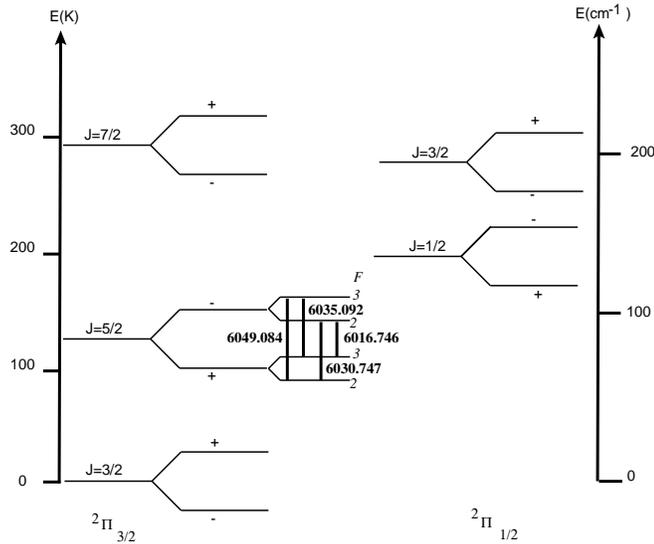
**Fig. 1.** The energy level diagram for the  ${}^2\Pi_{3/2}$  and  ${}^2\Pi_{1/2}$  ladders of the hydroxyl radical, OH. The lowest levels are shown. Transitions between the  $F = 3$  and  $2$  hyperfine levels give rise to the four 6 GHz lines
