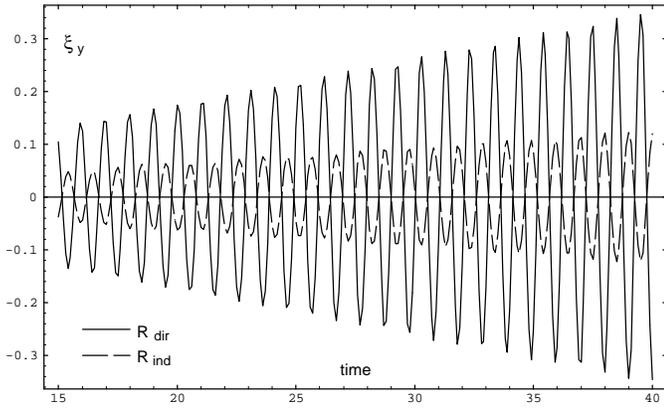
**Fig. 9.** The amplitude of  $\xi_y$  at the resonance as function of time for  $k_y = 2$  with the driving frequency  $\omega_d = 6.12$  for the direct and indirect driver.
