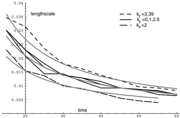
**Fig. 13.** The reduction of the length scale of the resonance in time with driving frequency  $\omega_d = 5.841$  for different values of  $k_y = 0, 1, 2, 2.5, 3.39$  corresponding with the different regions discussed in Paper I. The dark gray lines correspond to  $1/t$  fits.
