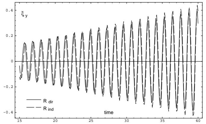
**Fig. 12.** The amplitude of  $\xi_y$  at the resonance as function of time for  $k_y = 2$  with the quasi-mode frequency as the driving frequency  $\omega_d = 6.12$  for the direct and indirect driver.
