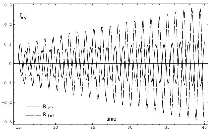
**Fig. 10.** The amplitude of  $\xi_y$  at the resonance as function of time for  $k_y = 2$  with the driving frequency  $\omega_d = 5.72$  for the direct and indirect driver.
