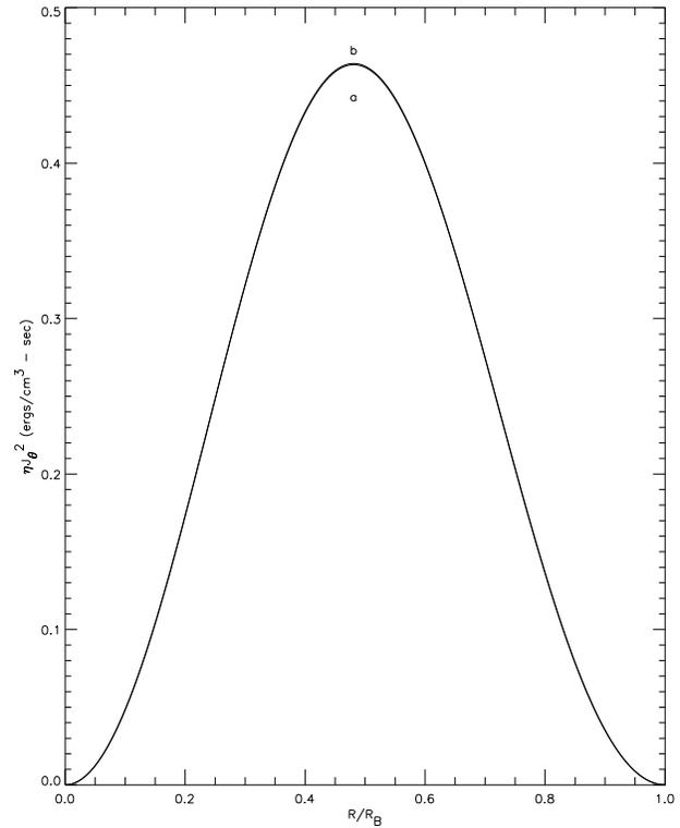
**Fig. 11.** Heating rate per unit volume vs.  $R/R_B$ . The scale height of  $\eta J_\theta^2$  is the same as for the pressure in Fig. 13. The average value of  $\eta J_\theta^2$  for solutions a and b is  $.222$  ergs-cm $^{-3}$ -sec $^{-1}$ .
