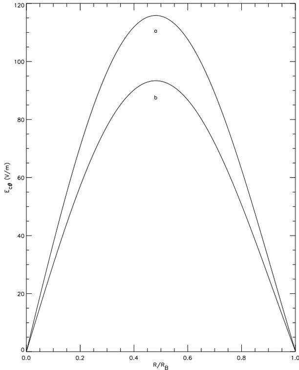
**Fig. 8.** Convection electric field vs.  $R/R_B$ . The scale height of  $E_{c\theta}$  is the same as for  $B$  in Fig. 5. The average values of  $E_{c\theta}$  for solutions a and b are 57.6 and 71.5  $\text{V}\cdot\text{m}^{-1}$ .
