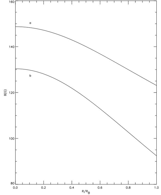
**Fig. 5.** Magnitude of the total magnetic field vs.  $R/R_B$ . The scale height of  $B$  is 1800 km for both solutions. The average values of  $B$  for solutions a and b are 134.1 and 108.8 G.
