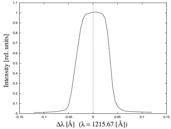
**Fig. 1.** Point Spread Function of the HST GHRS instrument (from Clarke et al. 1995).
