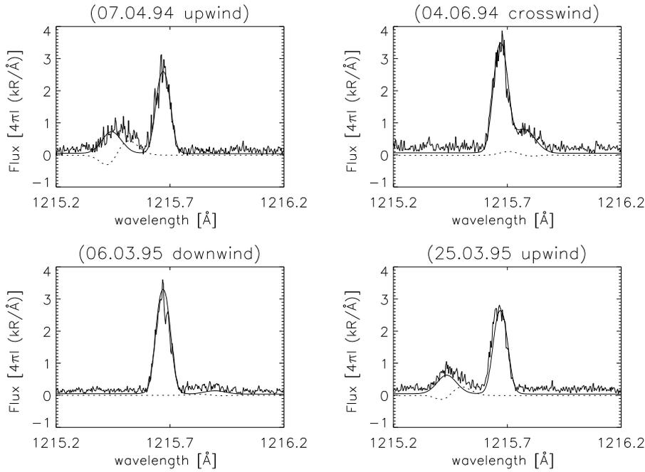
**Fig. 6.** Comparison of the HST data with the theoretical result (case 2). – calculated spectrum by the radiation transport model by Scherer & Fahr using a realistic solar profile; ····· difference of best data fit and calculated intensity ( $I_{\text{fit}} - I_{\text{theo}}$ ) see text.
