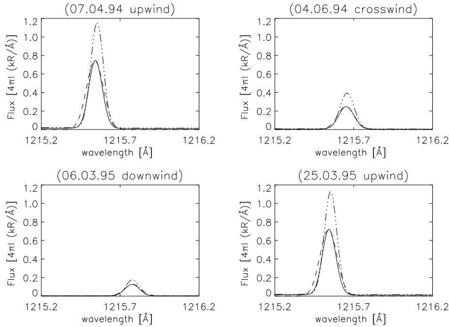
**Fig. 5.** Calculated spectra for alternative assumptions: - - - Voigt-profile with 30000 K; case 1: - · - · - radiation transport model by Scherer & Fahr using a flat solar profile and an optically thin approximation (details see text). case 2: - radiation transport model by Scherer & Fahr using a realistic solar profile, angle-dependent redistribution and self-absorption. The different cases are calculated for the four positions and view directions of the HST (see Table 1).
