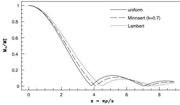
**Fig. 2.** Modulation function of the first harmonic as a function of the spatial frequency  $x$ , for a uniformly bright disk (solid curve), a Lambertian disk (dotted) and distribution following Minnaert's law with  $k = 0.7$  (dashed)
