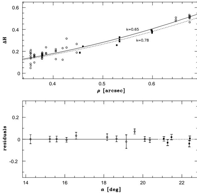
**Fig. 3.** Harmonics attenuation expressed on logarithmic scale (magnitude bias  $\Delta H$ ) for Hipparcos observations of minor planet (1) Ceres (top). Each point correspond to a transit of the planet across the field of view. The residuals (bottom) are calculated from a light scattering following Minnaert law, for two subsets in solar phase angle: circles,  $\alpha < 21^\circ$  and squares,  $\alpha > 21^\circ$ . Each point is a mean of successive transits
