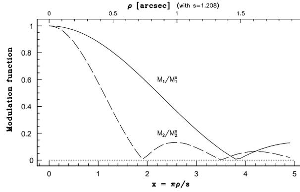
**Fig. 1.** Modulation function for the first two harmonics of a uniformly bright disc as a function of the spatial frequency  $x$ . The abscissa scale is also given in terms of apparent diameter for the Hipparcos main grid of period  $s = 1''.208$
