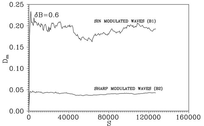
**Fig. 6.** Simulated values of the magnetic field diffusion coefficient  $D_m$  versus distance along the field line  $s$ . Results for the models B1 and B2 are presented for  $\delta B = 0.6$ . For 1-D model A the diffusion coefficient vanishes,  $D_m = 0$ .
