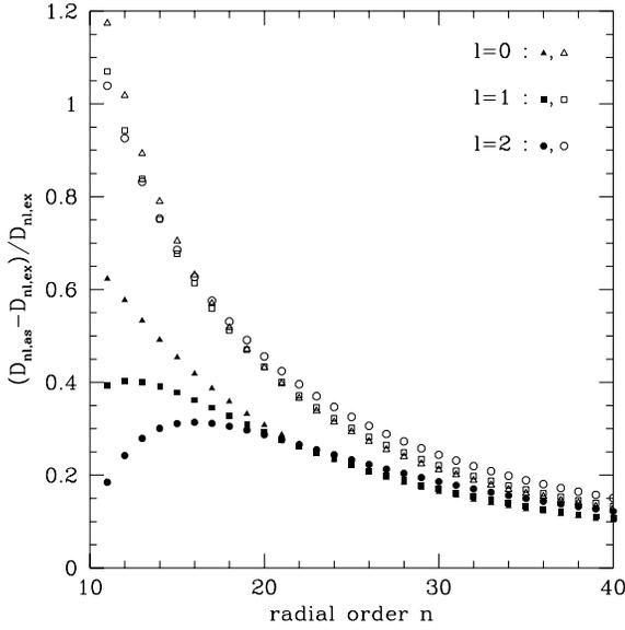
**Fig. 7.** Relative errors of the scaled frequency separations  $D_{n,\ell}$  obtained from the second asymptotic approximation of the eigenfrequencies for the degrees  $\ell = 0, 1, 2$  (solid symbols), for a polytropic model with index equal to 3. Relative errors of the scaled frequency separations determined by means of the usual asymptotic theory are shown for comparison (open symbols).
