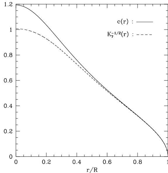
**Fig. 2.** Variation of the velocity of propagation of an acoustic wave modified by gravity and density stratification, in a polytropic model with index equal to 3. The variation of the isentropic sound velocity  $c(r)$  is also displayed for comparison.
