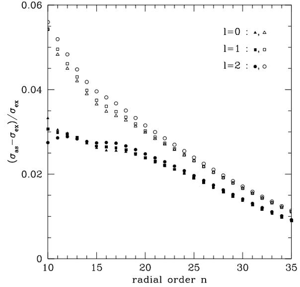
**Fig. 8.** Relative errors of the first asymptotic approximations of eigenfrequencies for the degrees  $\ell = 0, 1, 2$  (solid symbols), for a standard solar model. Relative errors of the first asymptotic approximations of eigenfrequencies determined by means of the usual asymptotic theory are shown for comparison (open symbols).
