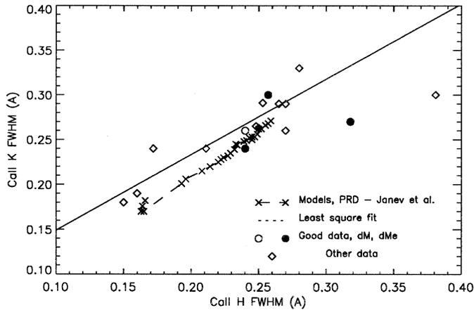
**Fig. 9.** CaII K line width as a function of CaII H line width. The line widths increase simultaneously and monotonically, but the K line remains about 30% broader because the optical depth in this line is a factor of two larger. Models agree with observations in this diagram, but Fig. 10 shows that except for intermediate activity stars, the width departs significantly from the empirical correlation
