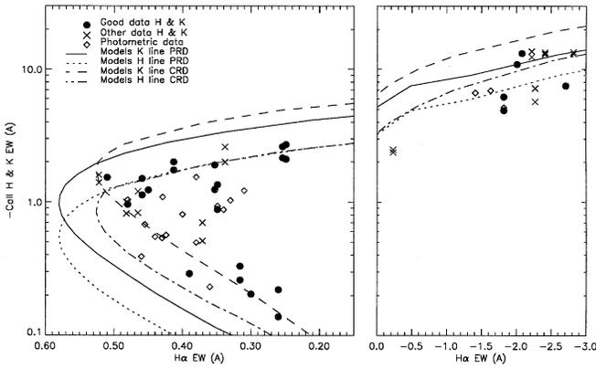
**Fig. 11.** Ca II line equivalent widths as a function of  $H_{\alpha}$  equivalent width for the models and the data. The large scatter in the data is attributed to surface inhomogeneities. The Calcium lines increase monotonically when  $H_{\alpha}$  goes through the low, intermediate and high activity domains as illustrated by the models. Hence, for a given  $H_{\alpha}$  equivalent width, the calcium lines can differentiate between the low and intermediate activity levels
