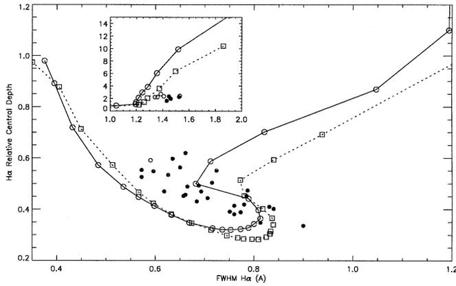
**Fig. 6.** We plot the  $H\alpha$  Relative Central Depth, i.e., the line center to continuum flux ratio, as a function of the FWHM (symbols have the same meaning as in Fig. 4b). This curve characterizes better the line profile shape than the EW vs. FWHM curve in Fig. 4. Comparison with the data shows that theoretical profiles are too deep for a given width and that an important factor, likely surface inhomogeneities, is responsible for the variety in the observed profile shapes.
