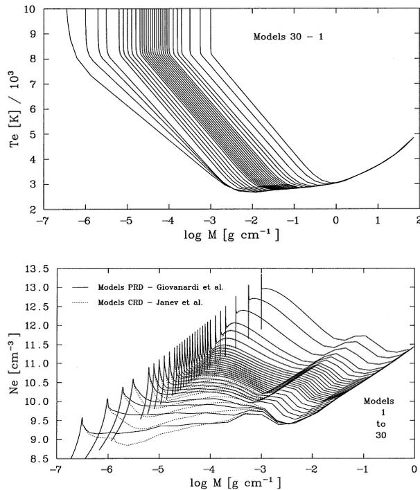
**Fig. 3.** Grid of model chromospheres for M1 dwarfs. Top panel, electron temperature as a function of column density. Lower panel, electron density as a function of column density (assuming hydrostatic equilibrium) for  $\text{Ly}\alpha$  calculated with two approximations: complete redistribution (CRD) and partial redistribution (PRD). These new models can reproduce several characteristics of the  $\text{H}\alpha$  and  $\text{CaII}$  lines as described in subsequent figures
