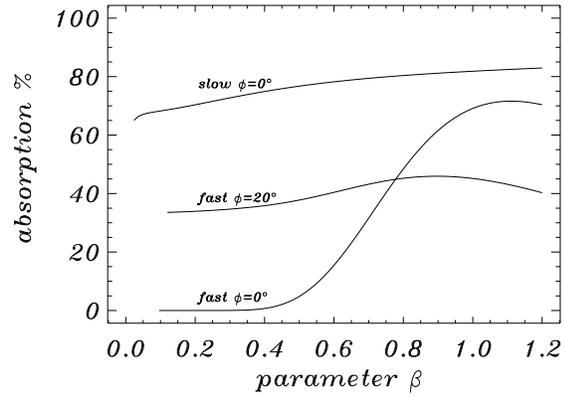
**Fig. 11.** The dependence of the absorption coefficient  $\mathcal{A}$  on the parameter  $\beta$  for fast and for slow MHD waves when:  $\omega = 6$  and  $\theta = 50^\circ$  and  $\phi$  as indicated.
