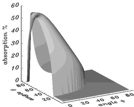
**Fig. 8.** The dependence of the absorption coefficient on the incident angle  $\theta$  and the azimuth angle  $\phi$  for fast MHD waves.
