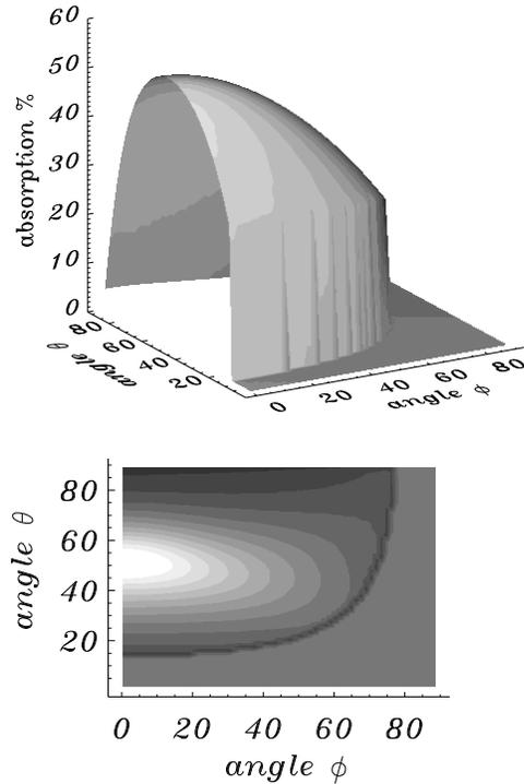
**Fig. 3.** **a** The dependence of the absorption coefficient on the incident angle  $\theta$  and the azimuth angle  $\phi$  for slow MHD waves. **b** The top view of the surface  $\mathcal{A}(\theta, \phi)$  showing the boundary of the computational domain. The dimensionless wave frequency is  $\omega = 0.8$ .
