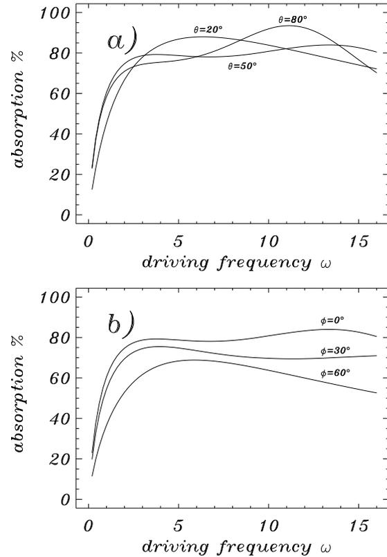
**Fig. 6a and b.** The dependence of the absorption coefficient  $\mathcal{A}$  on the wave frequency  $\omega$  for slow MHD waves for: **a**  $\phi = 0^\circ$  and **b**  $\theta = 50^\circ$  and other parameters as indicated.
