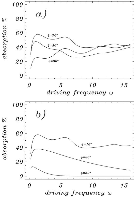
**Fig. 10a and b.** The dependence of the absorption coefficient  $\mathcal{A}$  on the wave frequency  $\omega$  for fast MHD waves for: **a**  $\phi = 10^\circ$  and **b**  $\theta = 70^\circ$  and other parameters as indicated.
