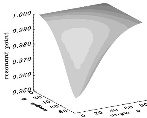
**Fig. 4.** The location of the cusp resonance depending on angles  $\theta$  and  $\phi$  for slow MHD waves with  $\omega = 0.8$
