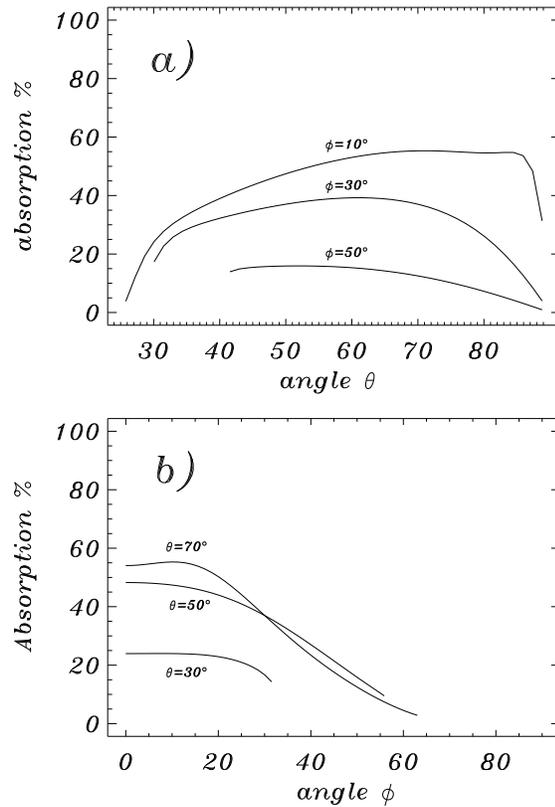
**Fig. 9a and b.** Absorption of fast MHD waves with the frequency  $\omega = 0.8$ . **a** The dependence of the absorption coefficient  $\mathcal{A}$  on the incident angle  $\theta$  at three indicated azimuthal angles  $\phi$ . **b** The dependence of the absorption coefficient  $\mathcal{A}$  on the azimuthal angle  $\phi$  at three indicated incident angles  $\theta$ .
