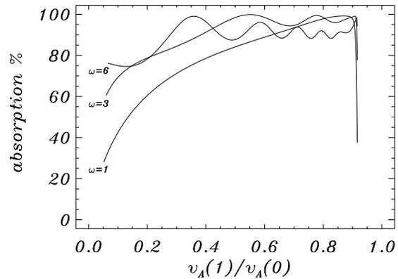
**Fig. 12.** The dependence of the absorption coefficient  $\mathcal{A}$  on the ratio of the Alfvén speeds  $v_A(1)/v_A(0)$  for slow MHD waves when:  $\beta = 0.6$ ,  $\theta = 50^\circ$  and  $\phi = 0^\circ$ .
