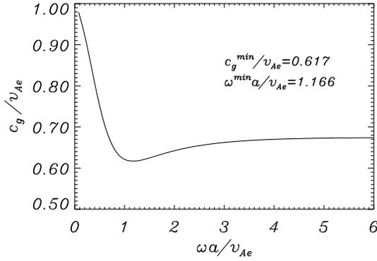
**Fig. 6.** The dimensionless group velocity  $c_g/v_{Ae}$  plotted as a function of dimensionless frequency  $\omega a/v_{Ae}$ , for the fundamental kink mode. A minimum in the group velocity occurs ( $c_g^{min}=0.617v_{Ae}$ ) for frequency  $\omega=1.166v_{Ae}/a$ . Impulsively generated kink waves will therefore show a wavepacket behaviour similar to that described by Roberts, Edwin & Benz (1984). No minima exist for the other modes.
