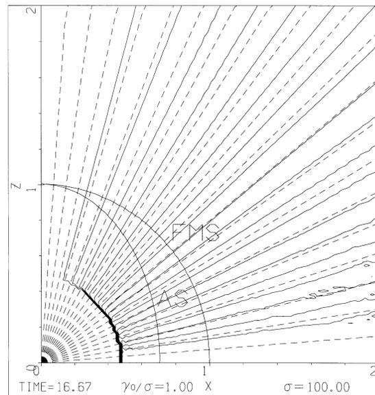
**Fig. 2.** The result of numerical simulation of the relativistic plasma flow when the Poynting flux is equal to the flux of the kinetic energy of plasma on the equatorial field line. The simulation was performed at the lattice dimension  $100 \times 100$ . The flow is stable. But the small vorticities of the poloidal electric currents appear more frequently.
