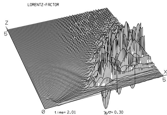
**Fig. 7.** The plot of Lorentz - factor of the plasma at the nonstationary flow of the Poynting flux dominated plasma. The nonstationarity of the flow leads to the acceleration of the plasma.
