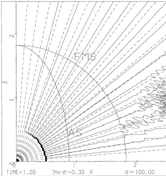
**Fig. 5.** The result of numerical simulation of the relativistic plasma flow at the same parameters as in the previous figure. The simulation was performed at the lattice dimension  $200 \times 200$ . The growth rate increased twice.
