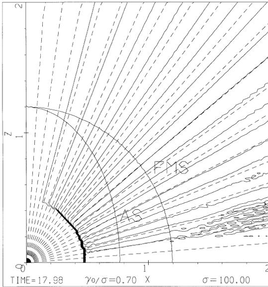
**Fig. 3.** The result of numerical simulation of the relativistic plasma flow when the Poynting flux slightly exceeds the flux of the kinetic energy of the plasma on the equatorial field line. The simulation was performed at the lattice dimension  $100 \times 100$ . The flow becomes nonstationary. There is a region near the equator where the stationary flow is unstable.
