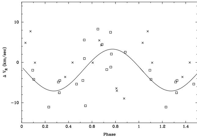
**Fig. 4.** Residuals in radial velocity for the 1951-1952 observations (open squares) and the 1906-1909 observations (crosses) plotted against the phase derived from the ephemeris of the eclipsing binary. The modulation has a  $3\sigma$  significance and has the correct phase.
