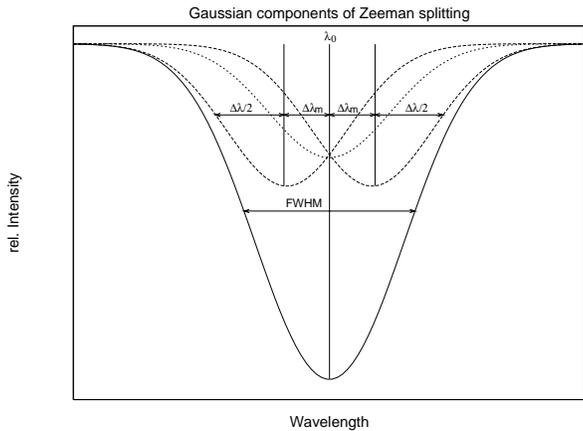
**Fig. 2.** Schematic Zeeman splitting with an intensity ratio for the components  $\sigma_{\pm}/\pi = 1.2$  which corresponds to an angle between the magnetic field and the line of sight of  $50^{\circ}$ .
