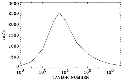
**Fig. 4.** The maximum value of the latitudinal velocity component in m/s as a function of the Taylor number for fixed angular velocity
