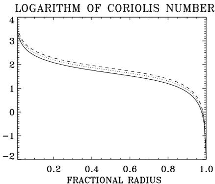
**Fig. 5.** The radial variation of the Coriolis number in a PMS star with 1.5 solar masses at the beginning of the contraction phase for different values of the mixing-length parameter. Solid line:  $\alpha_{\text{MLT}} = 1$ , dotted line:  $\alpha_{\text{MLT}} = 5/3$ , dashed line:  $\alpha_{\text{MLT}} = 2.4$
