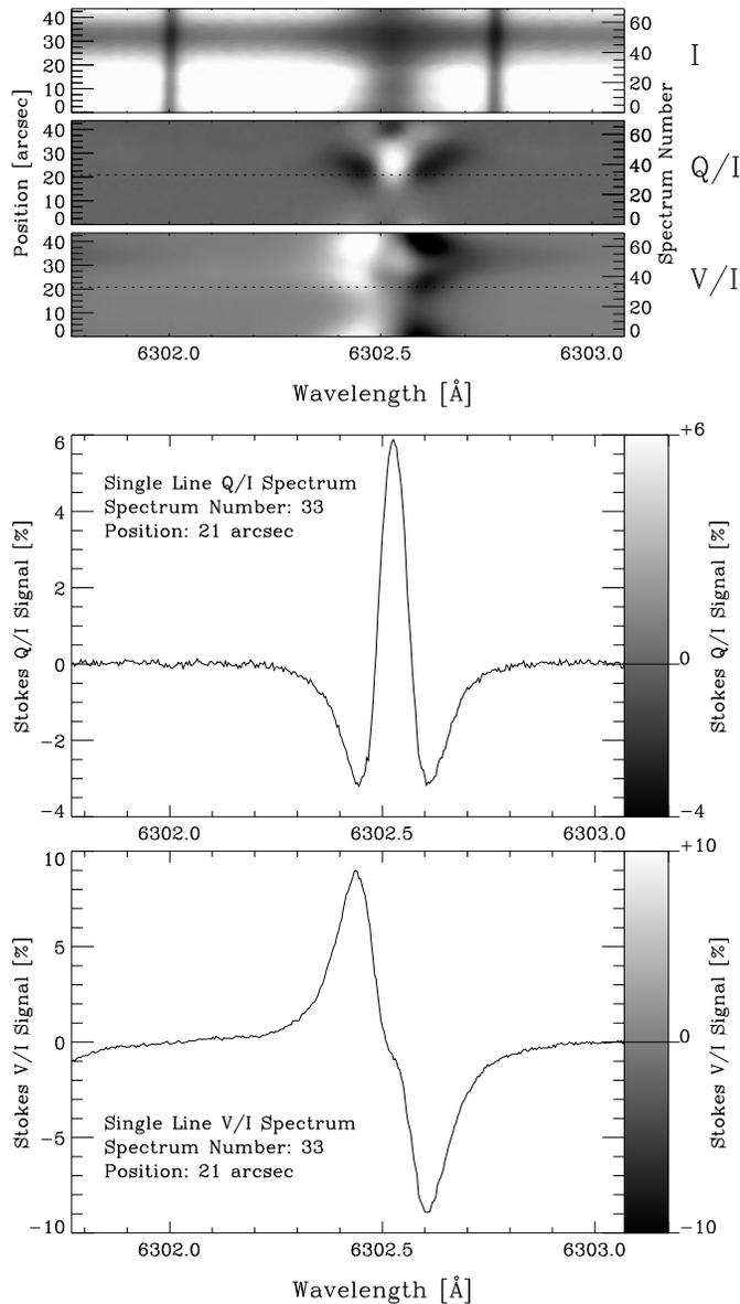
**Fig. 9.** Zeeman polarization of Fe I in a sunspot recorded at IRSOL in July 1996. Stokes  $I$ ,  $Q/I$ ,  $V/I$  have been recorded simultaneously. The spectra correspond to polarization images at position of 21 arcsec as indicated by the dotted line. The data have been averaged over 50 frames with 1 s integration time each. No Fourier filter or any other noise reduction technique has been applied. The gray-scales of the  $Q/I$  and  $V/I$  images are shown in the lower figure.
