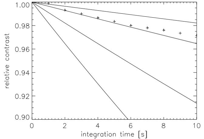
**Fig. 7.** Degradation of the linear polarization signal with integration time. 10 s of integration time corresponds to  $5 \times 10^5$  shifting cycles. The crosses indicate measured values. The curves have been calculated for different charge transfer inefficiencies  $\epsilon$  as explained in the text.  $\epsilon$  varies from  $10^{-8}$  (upper curve), to  $2 \times 10^{-8}$ ,  $5 \times 10^{-8}$ , and  $10^{-7}$  (lower curve).
