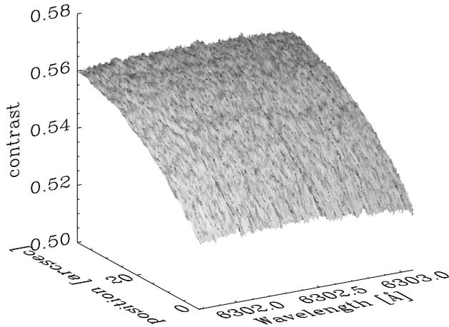
**Fig. 6.** Polarization gain table for Stokes  $Q/I$ , representing the Stokes  $Q/I$  calibration for the spectropolarimetric measurements in Fig. 9. The variation along the spatial direction arises from the sinusoidal mechanical stress distribution in the modulator (see Kemp 1969) that was placed before the entrance slit of the spectrograph.
