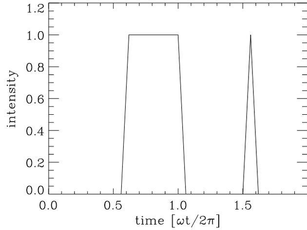
**Fig. 3.** Intensity of unmodulated light seen by the charge package  $q_3$  during one demodulation cycle (the ‘window function’).
