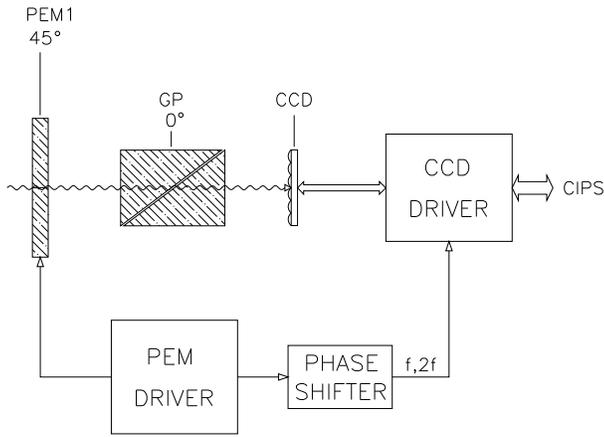
**Fig. 1.** Block diagram of the polarimeter. The polarization is modulated by a piezoelectric modulator (PEM1) followed by a Glan linear polarizer (GP). The CCD driver is connected to a control and image processing system (CIPS).
