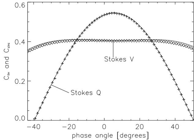
**Fig. 5.** Calculated (solid lines) and measured (crosses and diamonds) phase angle dependences of  $C_{\text{lin,max}}$  (pure Stokes  $Q$ ) and  $C_{\text{circ,max}}$  (pure Stokes  $V$ ). By adjusting the phase offset the measured curves have been shifted in the horizontal direction for optimum agreement with the theoretical curves.
