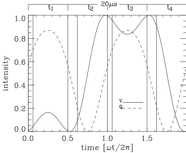
**Fig. 2.** Modulation functions for 100% linearly ( $Q$ ) or circularly ( $V$ ) polarized light. Stokes  $Q$  is modulated at  $2\omega$ , while Stokes  $V$  is modulated at  $\omega$ . At the beginning of each demodulation time interval  $t_{1,2,3,4}$  the charge packages are shifted by one pixel ( $0.6\mu\text{s}$ ) or two pixels ( $1.2\mu\text{s}$ ), according to the shifting scheme (see text).
