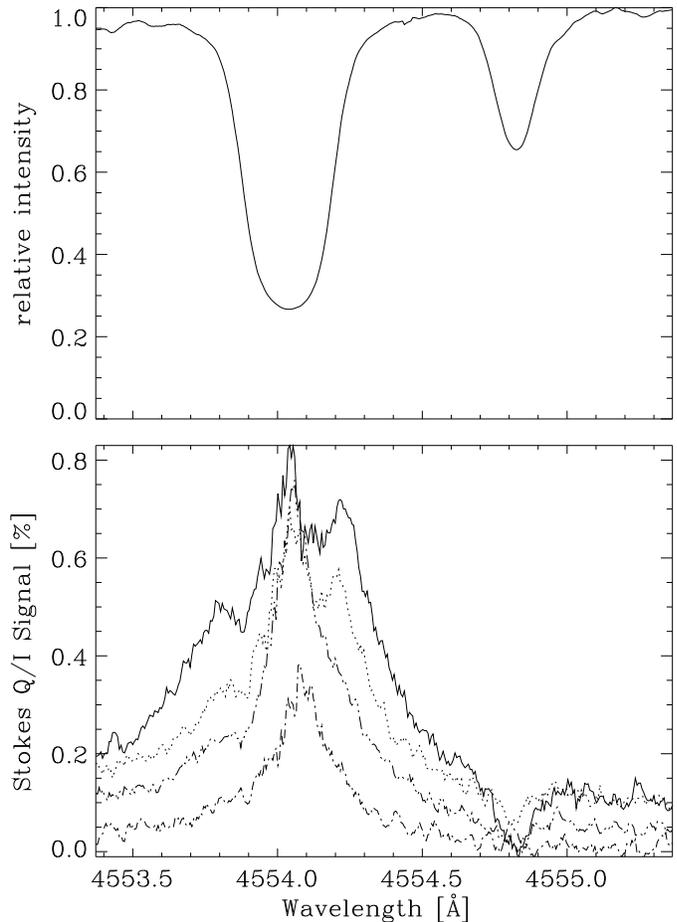
**Fig. 10.** Stokes  $I$  spectrum around 4554 Å with the Ba II line at 4554.0351 Å and the Cr I line at 4554.8229 Å and Stokes  $Q/I$  spectra for different distances from the solar limb. The polarization decreases with increasing heliocentric angles  $\theta$ , ranging from  $\mu = 0.05$ ,  $\mu = 0.1$ ,  $\mu = 0.15$ ,  $\mu = 0.2$ ,  $\mu$  being  $\cos \theta$ .
