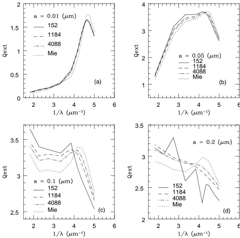
**Fig. 3a–d.** Extinction efficiencies ( $Q_{\text{ext}}$ ) for porous Graphite grains
