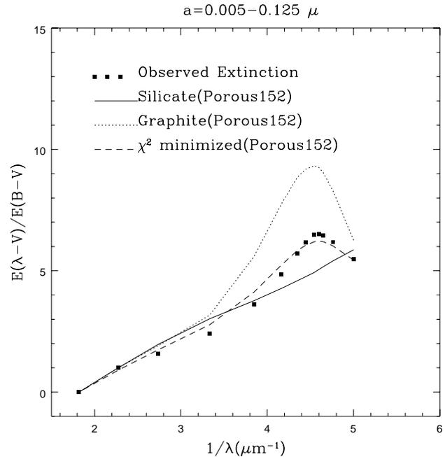
**Fig. 4.** Comparison of the observed interstellar extinction curve with the best fit model combination curve of porous silicate and graphite grains with the number of dipoles  $n=152$ .
