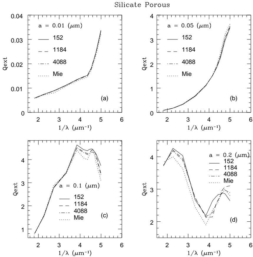
**Fig. 2a–d.** Extinction efficiencies ( $Q_{\text{ext}}$ ) for porous Silicate grains.
