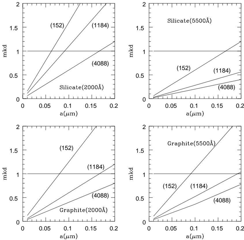
**Fig. 1.** Lattice dispersion relation  $mkd$  as a function of grain size at two wavelengths for the porous silicate and graphite grains.
