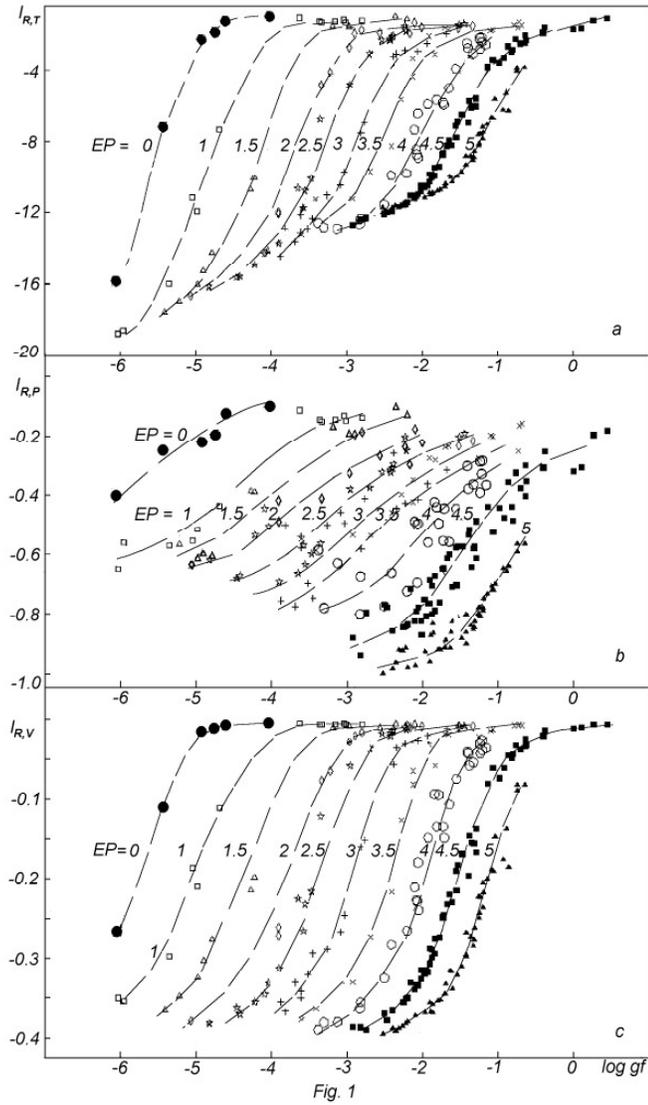
**Fig. 1a–c.** Indicators of the sensitivity of central depths of Fe I lines depending on the oscillator strengths  $\log gf$  and lower excitation potentials ( $EP$ , eV): **a** to the temperature; **b** to the gas pressure; **c** to the microturbulent velocity.
