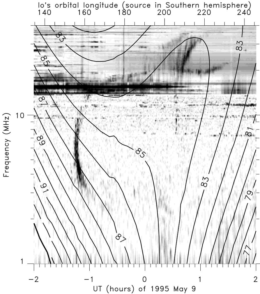
**Fig. 6.** Same as Fig. 5 but for the Io-D (LH polarized, or Southern hemisphere) emission. Note the magnetic anomaly (change in curvature of the iso-contour lines) and the (maybe coincidental) distortion of the arc shape emission.
