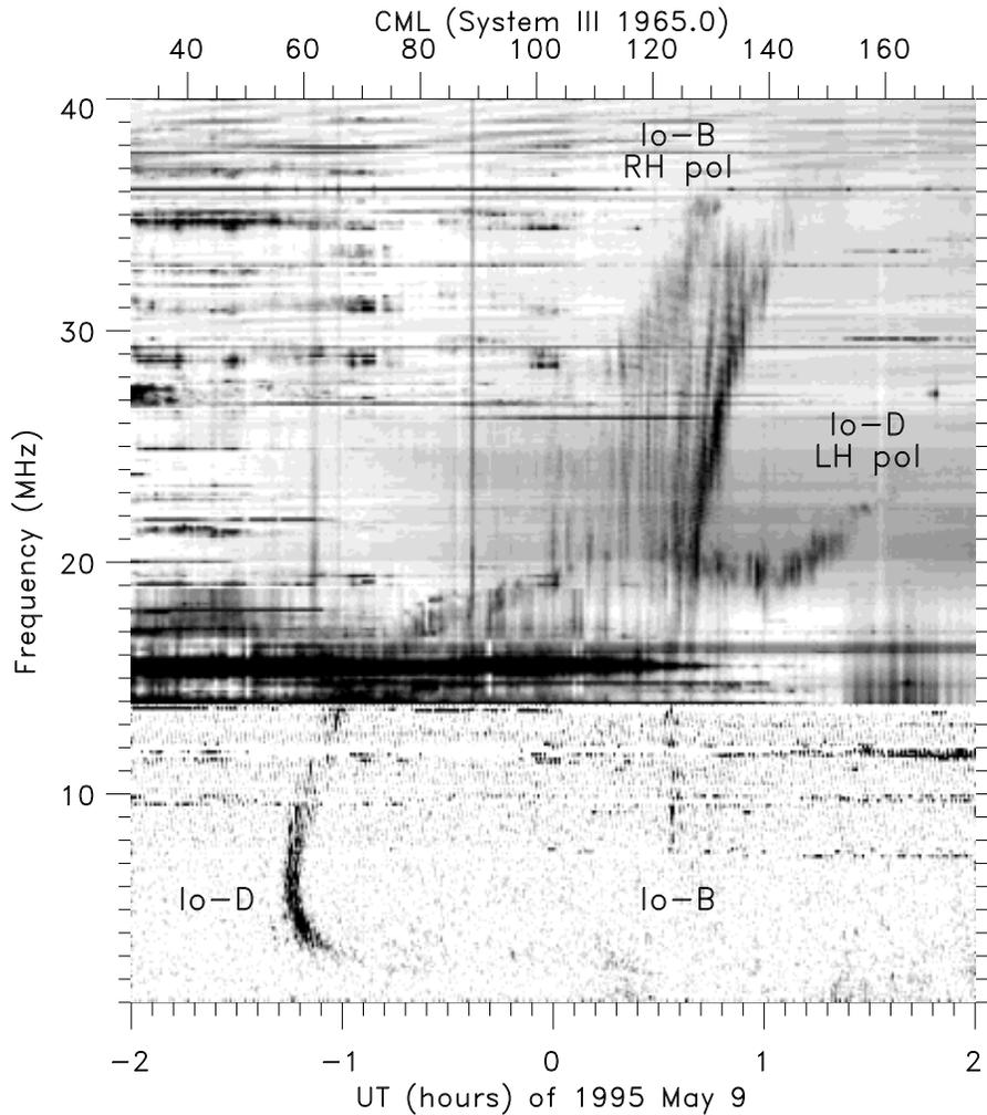
**Fig. 2.** Dynamic spectrum of the event of 1995, May 8/9<sup>th</sup>, displaying the complete beam pattern of the Io flux tube radiation. Two Io-controlled arc-shaped patterns are recorded, Io-B and Io-D, in opposite sense of circular polarizations. Both radiations are observed together during more than one hour, each emanating from different hemispheres. As in the previous event, the dynamic spectrum is the composition of two observations, from Nançay and Wind/WAVES.
