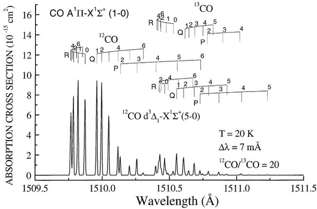
**Fig. 2.** Optically thin, calculated absorption spectrum of the CO  $A^1\Pi - X^1\Sigma^+$  ( $v'=1, v''=0$ ) band. The parameters used correspond to those obtained by the fit shown in Fig. 4
