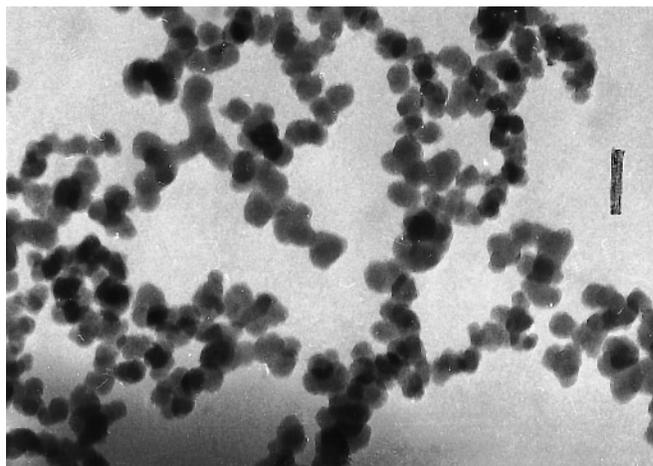
Fig. 1. Micrograph of an as-formed pyrolysis powder. Bar=100nm.
