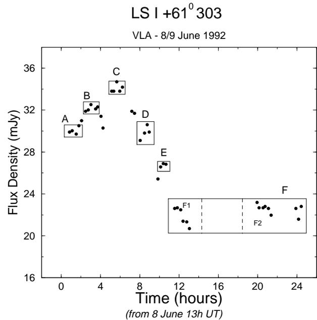
**Fig. 2.** Flux variations measured by the VLA during our VLB experiment, with boxes showing the different datasets used to make individual VLBI images during periods when the flux was roughly constant
