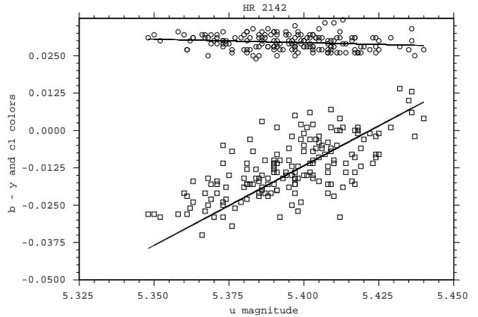
**Fig. 14.** The  $b-y$  ( $\square$ ) and  $c_1$  ( $\circ$ ) colors correlated with the  $u$  magnitude. Only data in one homogeneous photometric system (System 7) have been considered. Best linear fits given by Eqs. (8) are shown.
