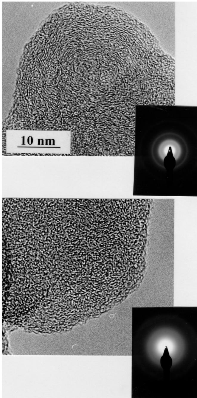
**Fig. 2.** High Resolution TEM images and Electron Diffraction Patterns (inserts) of infrared laser pyrolysis samples: concentric microtexture in sample B (top); amorphous phase in sample E (bottom)
