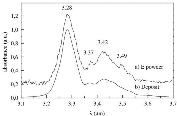
**Fig. 4.** C-H stretch region (3.1–3.6  $\mu\text{m}$ ) of the IR spectrum of a) powder E, b) the deposit, after linear background subtraction
