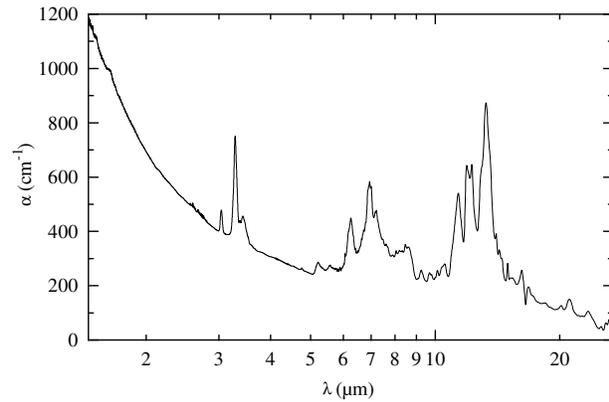
**Fig. 3.** Spectral absorptivity of deposited sample measured in the transmission mode in the 1.5-25  $\mu\text{m}$  range ( $\alpha = \ln(I_0/I)/d$ , where  $d=17 \mu\text{m}$  is the deposit thickness, and  $I$  the transmitted IR intensity)
