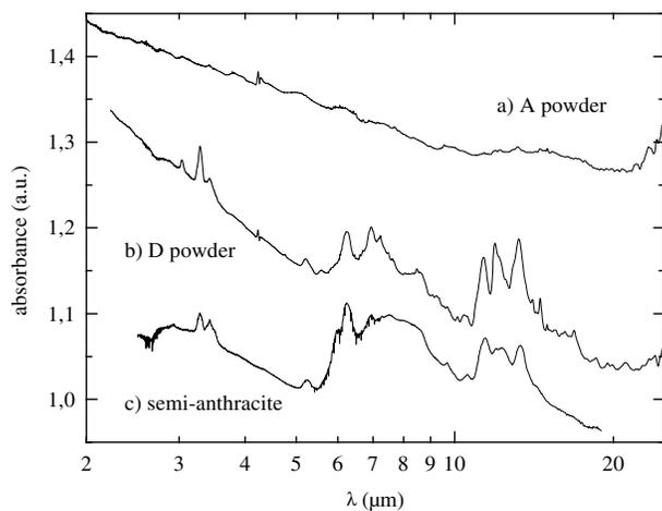
**Fig. 1.** DRIFT spectra recorded in the 2.5–25  $\mu\text{m}$  range. The curves refer to a) powder A, b) powder D (see Table 1 for synthesis conditions), c) semi-anthracite coal, presented here for comparison. Data are given as  $\log(1/R)$ . In all spectra a small contribution at 4.25  $\mu\text{m}$  due to  $\text{CO}_2$  present in the spectrometer has been subtracted
