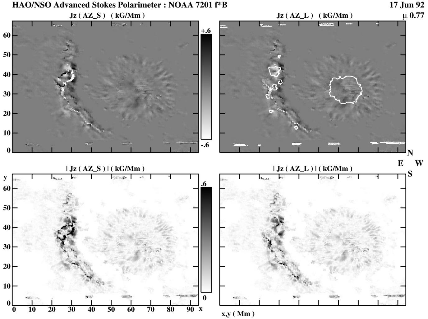
**Fig. 3.** Comparison of total vertical current for two alternative disambiguations. The lower row gives the absolute values. The white contour lines give umbra-penumbral transition boundaries.
