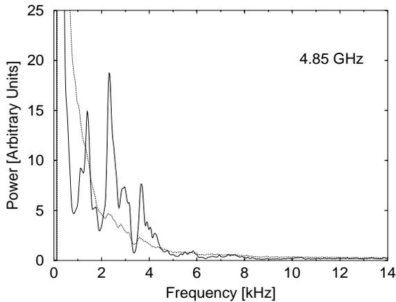
**Fig. 5.** Comparison between averaged power-spectrum (dotted curve) and ADP (solid line) of PSR B1133+16. The ADP shows strong maxima, only faintly visible in the power-spectrum.
