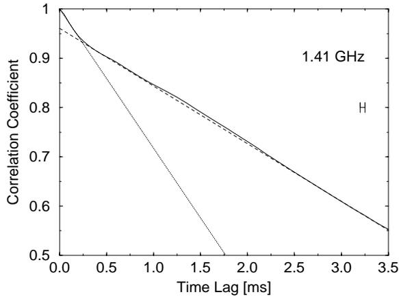
**Fig. 4.** Tangents to the averaged single pulse ACF of PSR B2016+28 at 1.41 GHz. The averaged ACF is represented by the solid line, the dotted and dashed line show the tangents to the short and longer parts of the ACF respectively. The error bar represents the sampling time of 50  $\mu\text{s}$ .
