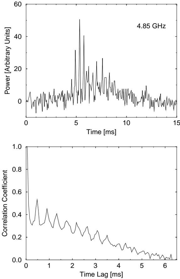
**Fig. 1.** An example of a single pulse of PSR B0950+08 with periodic microstructure and its ACF at 4.85 GHz. The time resolution is  $53 \mu\text{s}$ .
