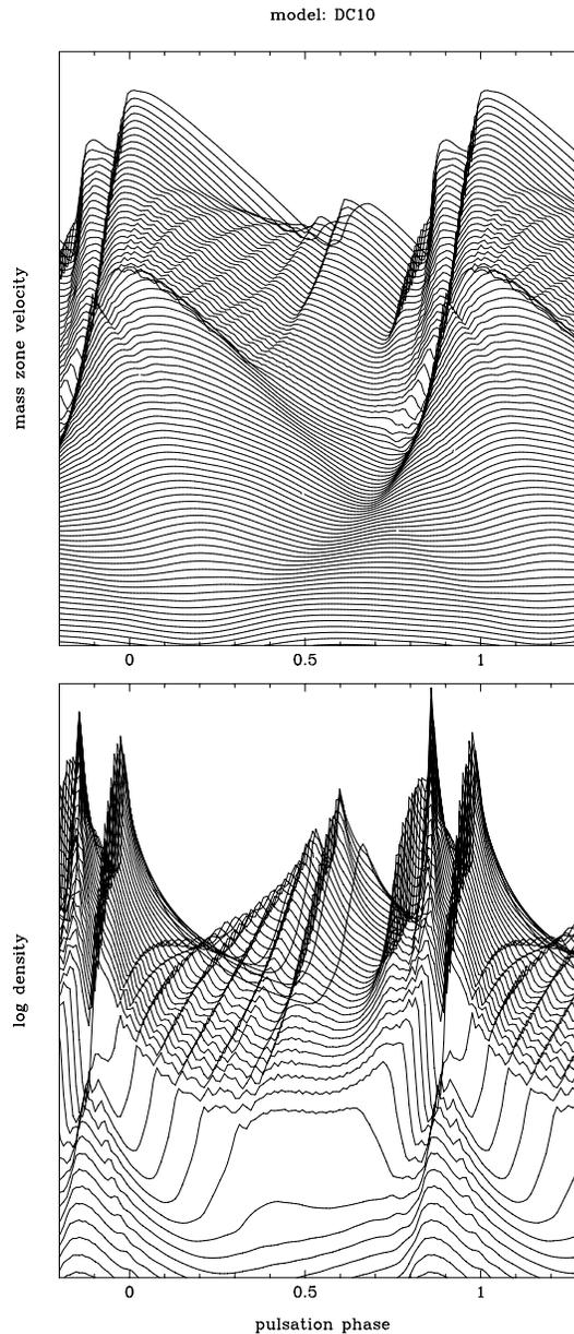
**Fig. 1.** Theoretical velocity (top) and density (bottom) variations with phase for different mass zones traced over 1.5 pulsation cycles of the classical Cepheid model  $\delta$  Cephei. The maximum and minimum radii occur about at phases 0.37 and 0.85 respectively (see FGB). Note that an arbitrary shift has been done between each mass zone to help the visibility. This explains the absence of velocity and density scales
