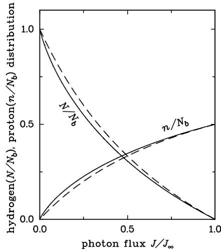
**Fig. 2.** The full curves show the hydrogen ( $N$ ) and proton ( $n$ ) densities in the layer as a function of  $J$  for the illustrative case  $\bar{c}_H = 4$ . The broken curves correspond to the asymptotic solution ( $\bar{c}_H \gg 1$ ).
