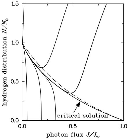
**Fig. 6.** The phase trajectories of the structure equation in the  $(N, J)$  plane. The broken curve is the locus of the minima of the integral curves. There is a unique critical solution which links the bottom of the layer ( $N = N_b, J/J_\infty = 0$ ) to the top ( $N/N_b = 1, J = 0$ ).
