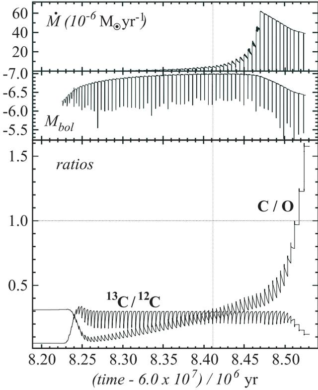
**Fig. 1.** AGB evolution of our  $6 M_{\odot}$  model with  $Z = 0.008$ . The top frame shows the mass-loss rate, the middle frame gives  $M_{bol}$ , and the lower frame presents the  $^{13}\text{C}/^{12}\text{C}$  and C/O ratios. The time when the mass-loss rate exceeds our critical value of  $5 \times 10^{-6} M_{\odot}/\text{yr}$  is shown as a vertical line. The horizontal line corresponds to C/O=1
