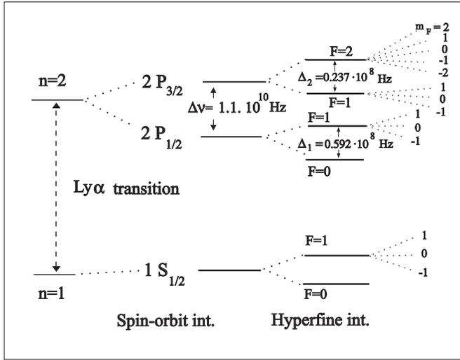
**Fig. 2.** The structure of the 1s-2p levels in hydrogen. Both spin-orbit and hyperfine interaction will cause a splitting of levels. The degenerate sub-states  $m_F$  of the hyperfine levels  $F$  is shown together with the size of the frequency separation caused by the two interaction mechanisms.
