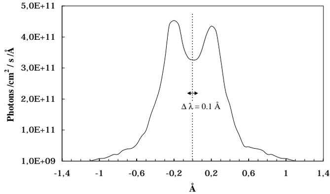
**Fig. 3.** The wavelength profile of the sun's Ly $\alpha$  line at 1 AU from the sun (adapted from Lemaire 1978). The profile is centered around the wavelength 1215.67 Å. Inserted in the figure is the FWHM  $\Delta\lambda$  for a Doppler profile corresponding to a gas of temperature 8000 K. The wavelength separation between the two P-states is 0.005 Å.
