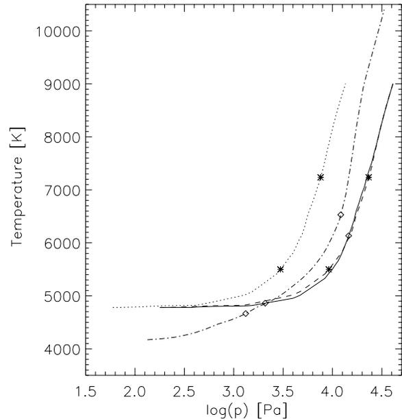
**Fig. 2.** Temperature versus pressure for various models. Solid: temperature of the atmosphere surrounding the flux tube; dashed: temperature in the flux tube, where the pressure is the total pressure, i.e., the sum of the gas and magnetic pressure; dotted: temperature versus gas pressure in the flux tube; dash-dotted: VALC model extended to deeper layers by model of Spruit. The asterisks and diamonds have the same meaning as in Fig. 1.
