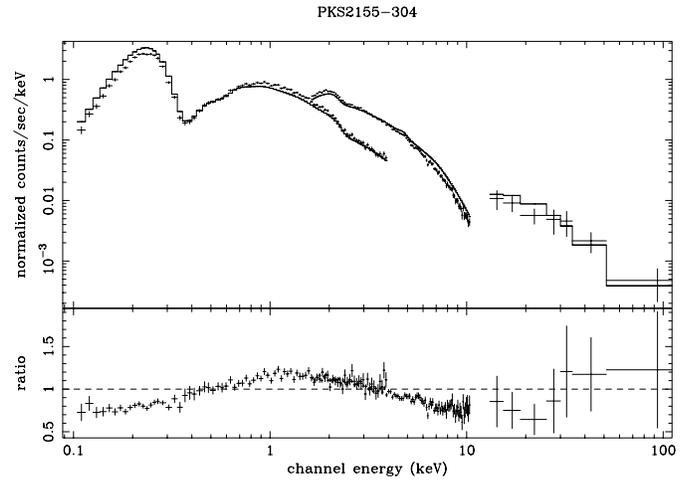
**Fig. 2.** Fit to a power law spectrum. The residuals from the best fit model clearly show spectral curvature up to 10 keV and an excess above 10–20 keV
