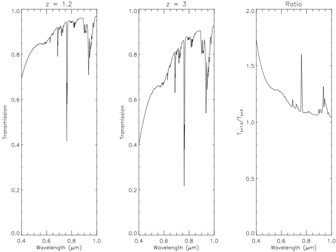
**Fig. 1.** Left and center panels: Transmission of the Earth atmosphere as computed using the LOWTRAN radiative transfer code at airmasses  $z = 1.2$  and  $z = 3$ . Right panel: Ratio between  $T_{z=1.2}$  and  $T_{z=3}$ .
