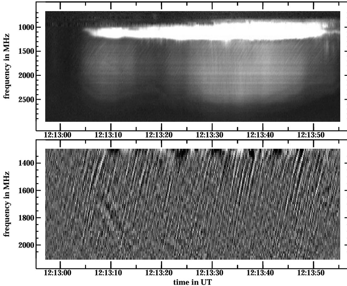
**Fig. 1.** *Top:* Spectrogram of a decimetric type IV burst observed with the Phoenix radio spectrometer of ETH Zurich on March 20, 1993. The preburst background has been subtracted, and the greyscale is logarithmic. *Bottom:* The intermediate drift bursts have been enhanced by subtracting a gliding average in frequency and time.
