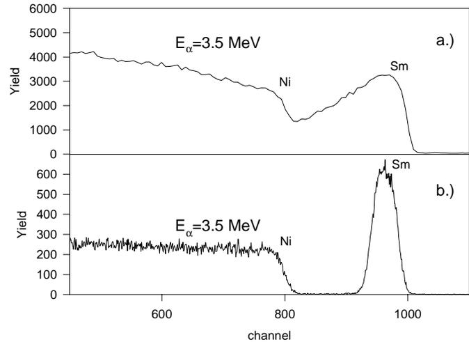
**Fig. 1a and b.** RBS spectra from (a) Sm oxide (beaded surface), and (b) metallic Sm targets on nickel backing
