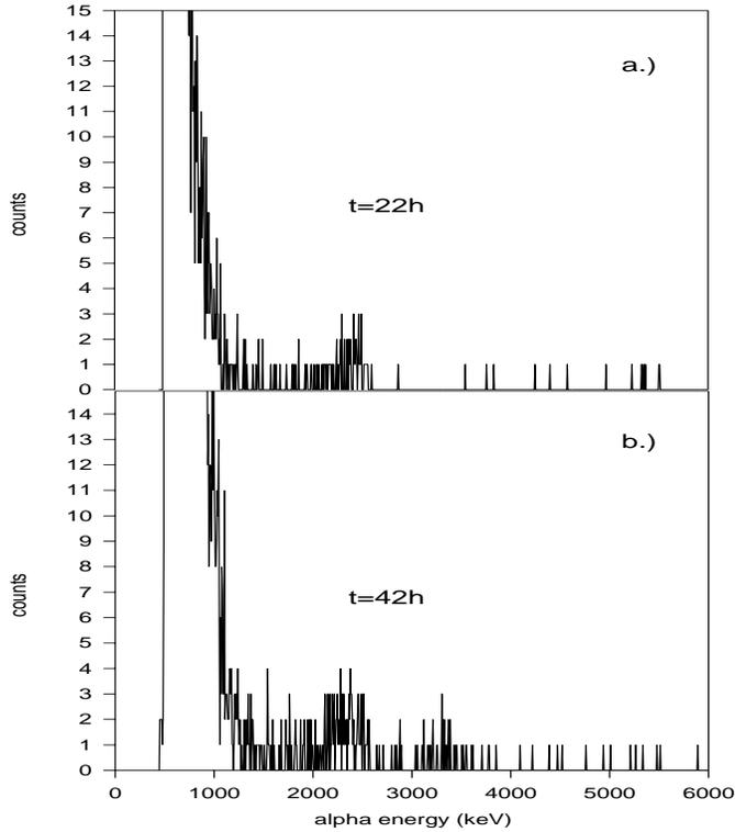
**Fig. 2a and b.** The  $\alpha$ -particle spectra from a target (a) before and (b) after irradiation
